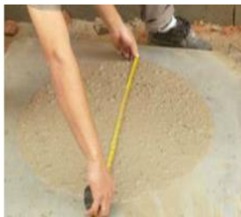
Figura 12.2 Teste de Slumpflow.
